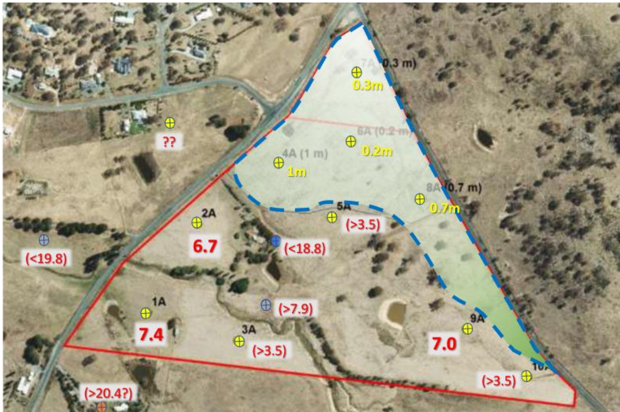
Figure 4-6: Depth to competent bedrock. Shaded area marked where bedrock is less than 3 m below ground. Numbers in brackets inferred from bore construction records.
