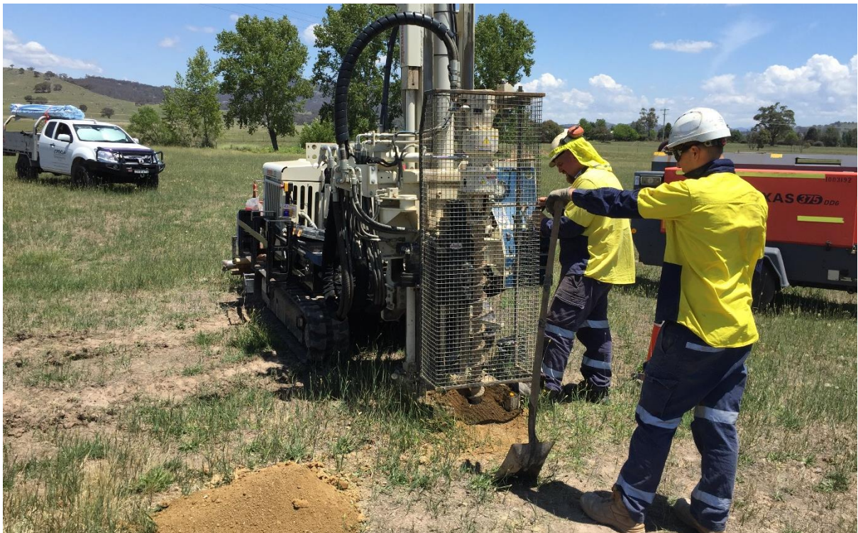
Figure 4 – Drilling borehole MW02B. Boreholes were excavated using a solid stem flight auger attachment from 0.5m bgl until auger refusal in bedrock, below which, deeper boreholes (MW02B and MW09B) were drilled into bedrock using an air hammer methods.
